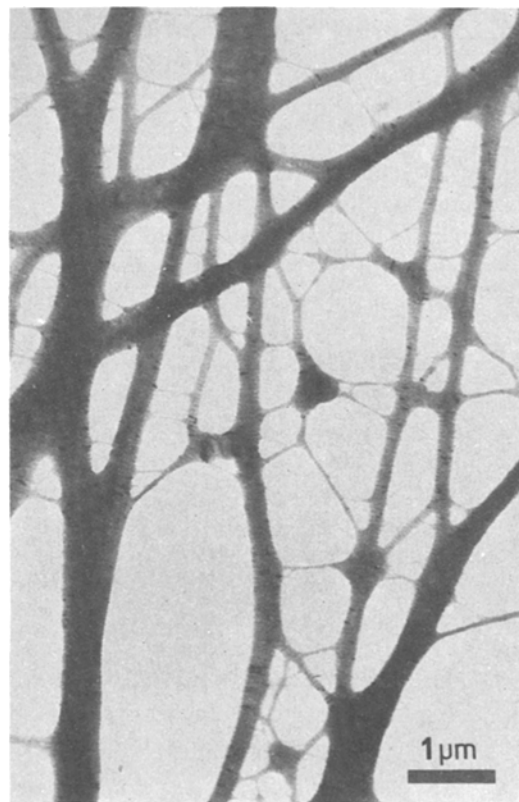
Figure 3 TEM of Marlex shish-kebabs heat-treated at 130° C for 5 min. The elementary fibrils have formed dense aggregates with a fine surface striation of 40 nm.
